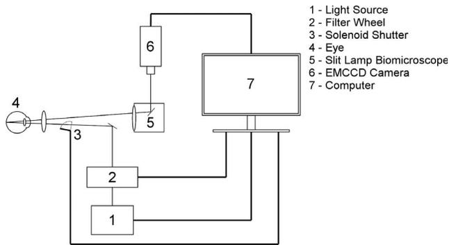
**FIGURE 1.** Schematic diagram of the optical imaging system for simultaneous measurement of retinal vascular diameter and oxygen saturation before and during light flicker stimulation. *Thick lines* represent physical connections between system components and *thin lines* represent the optical path.
